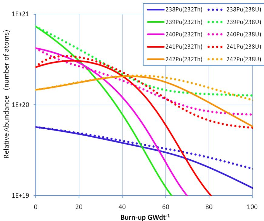
**Fig. 1.7:** Relative atom populations for plutonium isotopes in 7% plutonium enriched PWR using thorium and  $^{238}\text{U}$  fuel platforms
