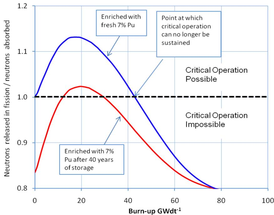
**Fig. 1.2:** Neutron economy versus burn-up for a 7% plutonium enriched MOX PWR using fresh plutonium and plutonium stored for 40 years
