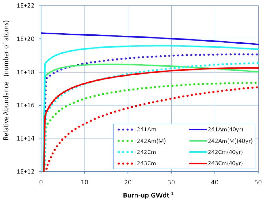
**Fig. 1.5:** Relative atom populations for a 7% plutonium enriched MOX PWR using fresh plutonium and plutonium stored for 40 years
