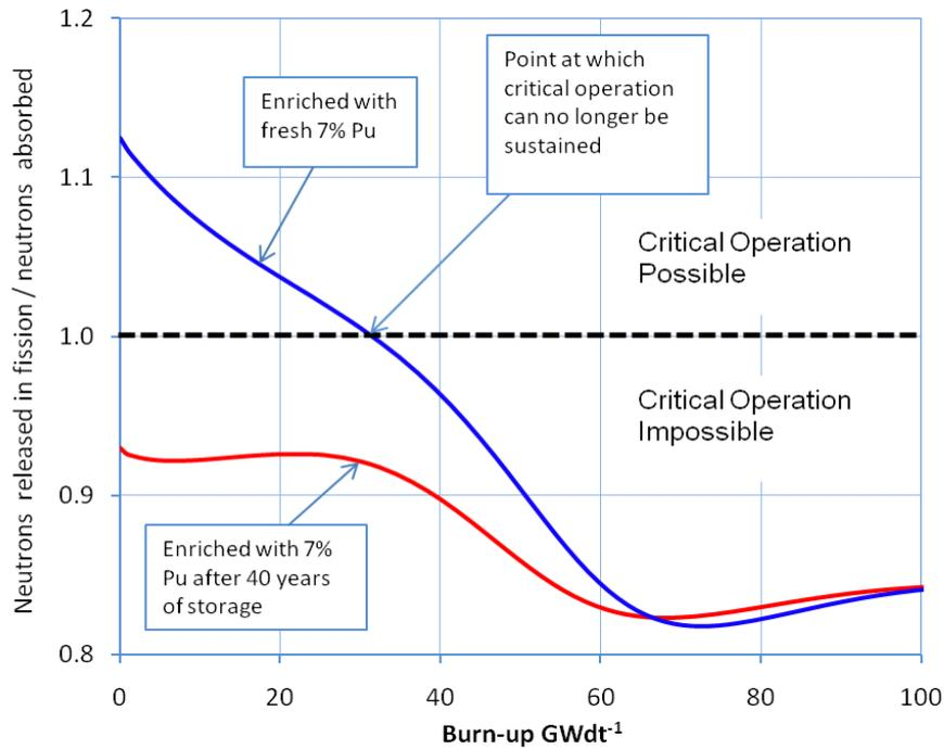
**Fig. 1.4:** Neutron economy versus burn-up for a thorium fuelled, 7% plutonium enriched MOX PWR using fresh plutonium and plutonium stored for 40 years
