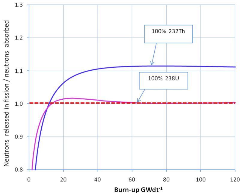
**Fig. 1.3:** Neutron economy ratio versus burn-up for 100% <sup>232</sup>Th and 100% <sup>238</sup>U fuel platforms in the thermal spectrum
