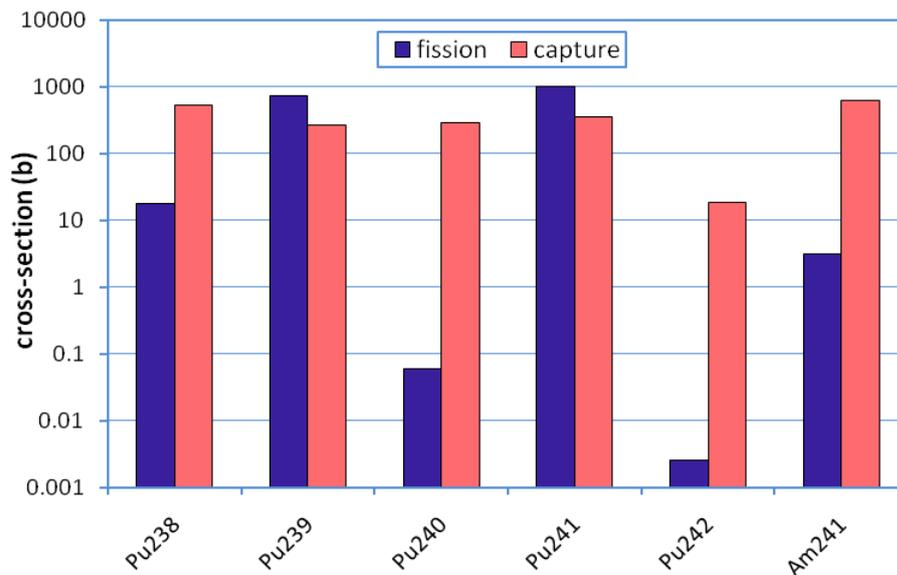
**Fig. 1.1:** One-group effective capture and fission cross-sections for selected nuclides in the thermal spectrum
