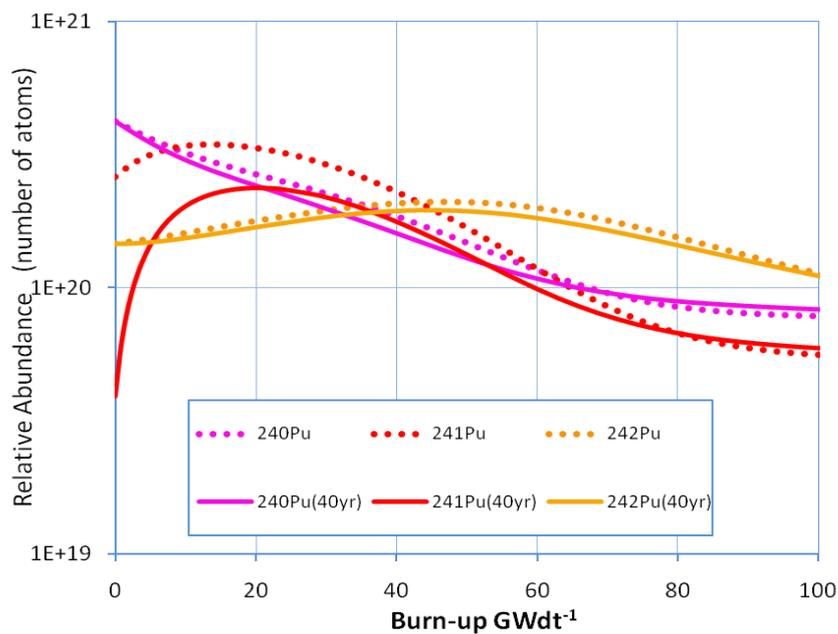
**Fig. 1.6:** Relative atom populations for <sup>240</sup>Pu, <sup>241</sup>Pu and <sup>242</sup>Pu using a 7% plutonium enriched MOX PWR for fresh plutonium and plutonium stored for 40 years
