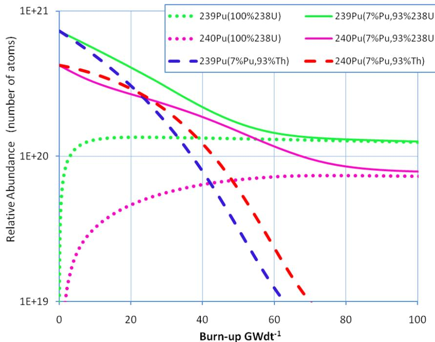
**Fig. 1.8:** Relative atom populations for plutonium isotopes in 7% plutonium enriched, pure  $^{238}\text{U}$  and enriched thorium PWR's
