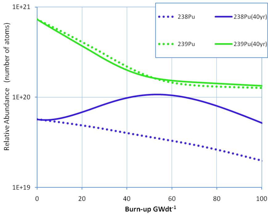
**Fig. 1.6:** Relative atom populations for <sup>238</sup>Pu and <sup>239</sup>Pu using a 7% plutonium enriched MOX PWR for fresh plutonium and plutonium stored for 40 years
