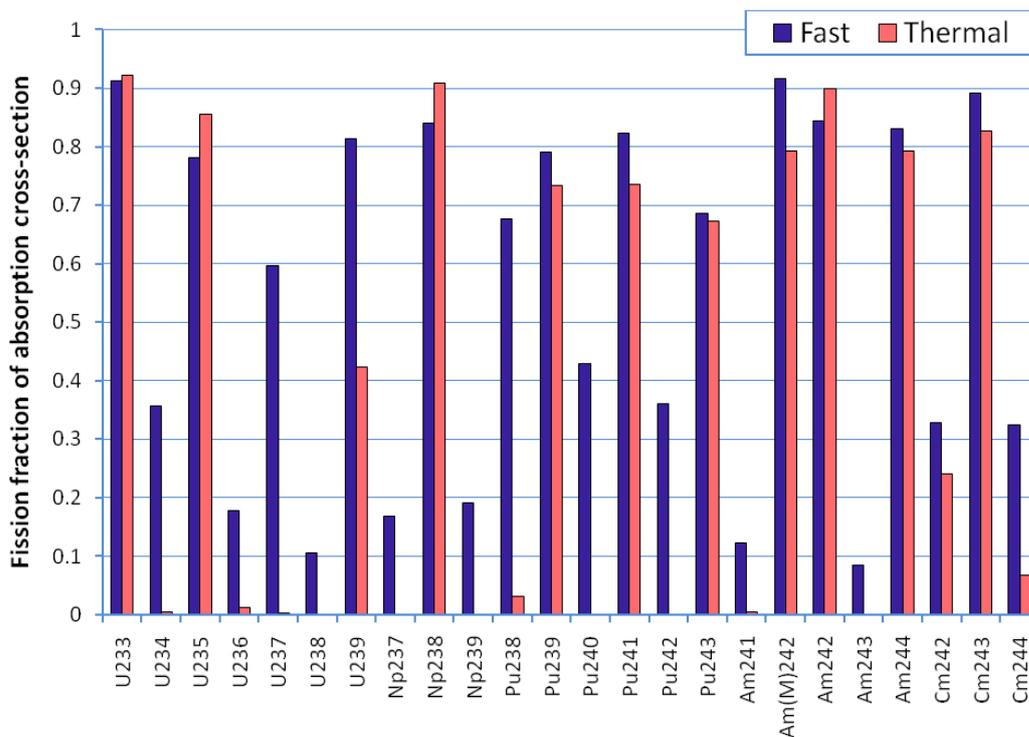
**Fig. 1.9:** Probability of fission as a fraction of the total neutron absorption cross-section for selected nuclides
